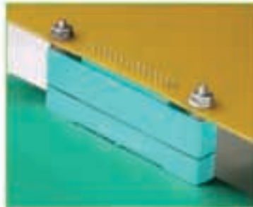
MB to I/O-P Mating Parallel Boards
